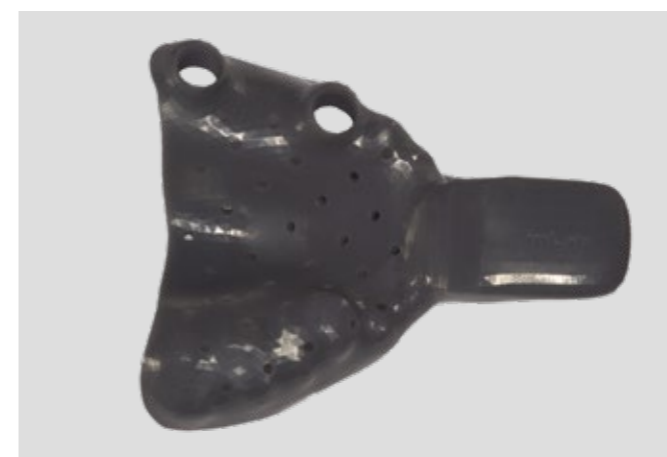
The design created with the inLab CAD SW was produced using a 3D printer.
