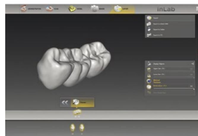
Afterwards, the restoration is ready to be exported. In this case the inLab MC X5 milling unit (Dentsply Sirona) was used. The case can also be exported into a STL format in order to utilize other open production units.
